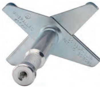
KD-CM16P Ceiling Frame Mount w/ Male 5/8" Spigot Adapter W 90g The Kupo Ceiling Frame Mount with Male Spigot Adapter is designed to attach to the metal frame which supports your ceiling tiles. This ceiling clip bracket mount has a 5/8" male stud that accepts lighting fixtures or any compatible 5/8" receiver accessory. Additional 1/4"-20 female thread on the top of baby pin also provides a great mounting solution for a Video/ Audio transmitter.
