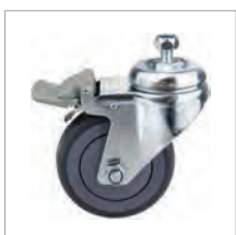
KC-100 Caster for 481 Stand Dia.: 100mm w/brakes and M10 attachment (17.5mm length) Set for three
