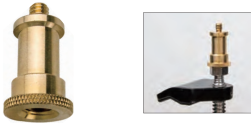
KS-073 Adapter Stud 3/8"-16F & 1/4"-20M W 40g Solid brass made 5/8" adapter stud with 3/8"-16 female thread is designed to convert an accessory with 3/8"-16 male threads to an industry-standard 5/8" stud to support equipment such as light fixtures. The stud is topped with 1/4"-20 male threads for additional mounting options.
