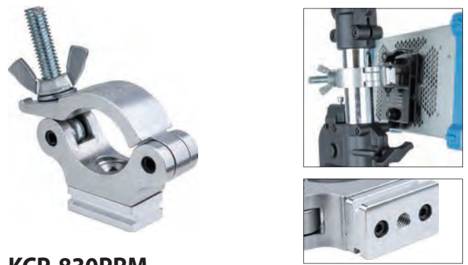
KCP-830PRM 2" Half Coupler for Skypanel PSU Mounting W 370g Aluminum made coupler for 2" comes with a CNC aluminum plate which allows Arri PSU Rail Mount Adapter to be effortlessly slid on. A great mounting solution for supporting the power supply unit on any 2" tube.
