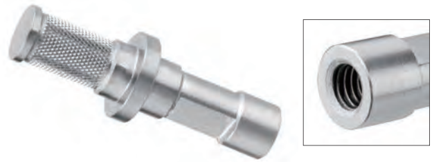
KS-151 Double Stud 16 to 17mm Adapter W 95g Made by solid steel, this double stud features a knurled neck on one side for the maximum friction and one milled flat on the other to avoid rotating while mounted inside a 5/8" baby receiver. Additional 3/8"-16 female threaded is tapped for connecting with a variety of accessories for video and lighting.
