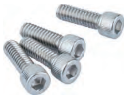
KS-294 1/4"-20 Stainless Steel Hex Socket Screw 3/4"(L)(Set of 4) W 16g
