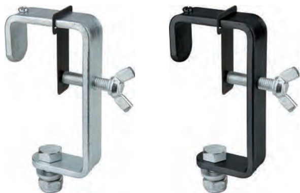
C-02N-P / C-02BN-P Clamp W 0.39kg ↓ 40kg Wing Bolt / M12 Bolt & Nylon nut: yes / Protective tab: yes
