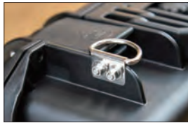
Enlarge the hole with 5.2mm twist drill bit.
