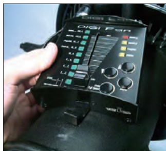
Switch for local or DMX operation mode.
