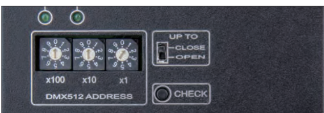
“Zero” switch is the initial aperture position where it can be set at fully closed or open as default. Check button is the self-examination function to inspect the unit works or not.
