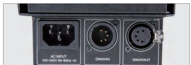
IEC and standard 5pin XLR receptacles neatly position at chassis atop.
