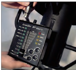
Multi functional control box for Manual, DMX and Program setting.
