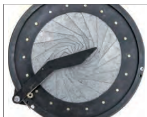
18-leave Iris for dia. 100mm aperture (with fully close shutter).
