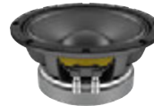
No. 12602518 LAVOCE WAF082.00 8" Woofer Ferrite Magnet Aluminium Basket Driver 200 W AES, 8 ohms, 95.5 dB, 80-3000 Hz
