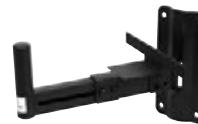
No. 60004620 OMNITRONIC Wall-Mounting XY for Speakers Fixation with clamp area (130-255 mm), movable & tiltable, max. load 25 kg
