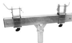
No. 59007082 EUROLITE TAH-35L-A2 Truss Adapter for STC-550 Adapter from 150 to 545 mm, 54 mm pin, max. load WLL 500 kg
