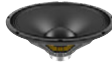
No. 12602619 LAVOCE WSN152.50 15" Woofer Neodymium Magnet Steel Basket Driver 250 W AES, 8 ohms, 97 dB, 45-3000 Hz
