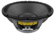
No. 12602535 LAVOCE WAF154.02 15" Subwoofer Ferrite Magnet Aluminium Basket Driver 800 W AES, 8 ohms, 96 dB, 40-1000 Hz
