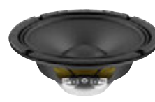
No. 12602610 LAVOCE WSN061.52 6.5" Woofer Neodymium Magnet Steel Basket Driver 125 W AES, 8 ohms, 94.5 dB, 90-5000 Hz
