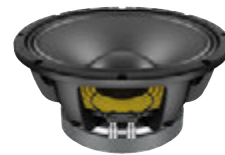
No. 12602530 LAVOCE WAF123.00 12" Woofer Ferrite Magnet Aluminium Basket Driver 500 W AES, 8 ohms, 99.5 dB, 50-2500 Hz
