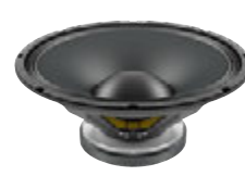
No. 12602533 LAVOCE SSF153.00 15" Subwoofer Ferrite Magnet Steel Basket Driver 400 W AES, 8 ohms, 97 dB, 45-2000 Hz
