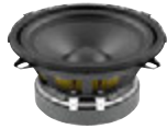
No. 12602511 LAVOCE WSF051.02 5" Woofer Ferrite Magnet Steel Basket Driver 60 W AES, 8 ohms, 91.5 dB, 100-5000 Hz
