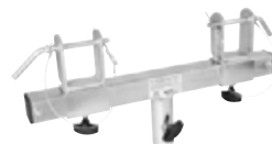
No. 59007079 EUROLITE TAH-35M Truss Adapter, large Adapter from 120 to 350 mm, 36 mm stand sheath, max. load WLL 300 kg
