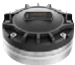
No. 12602815 LAVOCE DN10.17T 1" Compression Driver Neodymium Magnet 55 W AES, 8 ohms, 107 dB, 1200-18000 Hz
