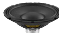
No. 12603211 LAVOCE NBASS10-20 10" Bass Guitar Woofer Neodymium Magnet Steel Basket Driver 150 W AES, 8 ohms, 96 dB, 50-5000 Hz
