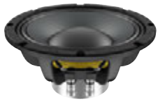
No. 12602613 LAVOCE WAN082.50 8" Woofer Neodymium Magnet Aluminium Basket Driver 250 W AES, 8 ohms, 94 dB, 75-2000 Hz
