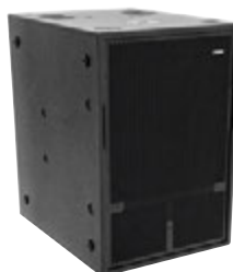
No. 11041142 PSSO K-211 Subwoofer 1600W Pro PA horn-loaded sub, 21" woofer, 1600 W RMS, 4 ohms
