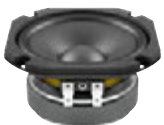
No. 12602919 LAVOCE FSF041.00 4" Fullrange Ferrite Magnet Steel Basket Driver 40 W AES, 8 ohms, 88 dB, 100-18000 Hz
