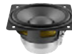
No. 12602912 LAVOCE FSN020.71F 2" Fullrange Neodymium Magnet Steel Basket Driver 15 W AES, 8 ohms, 87 dB, 200-20000 Hz
